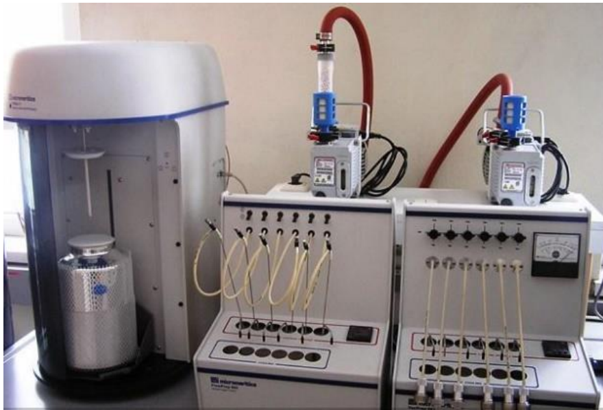
Figure 4.5-5: BET instrument to investigate the specific surface areas and pores diameter
