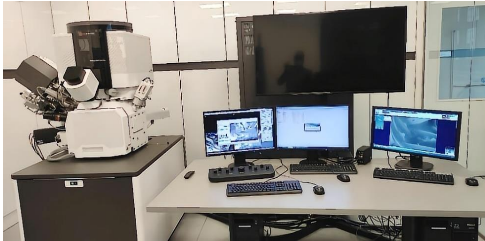
Figure 4.5-3: SEM and EDS instruments to investigate the morphology and the particles sizes
